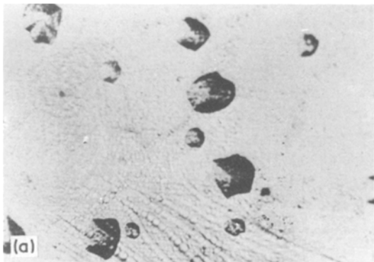
Figure 4 Production of hillocks by conc. H 2 SO 4 . Temperature of etching 30° C; × 175.
